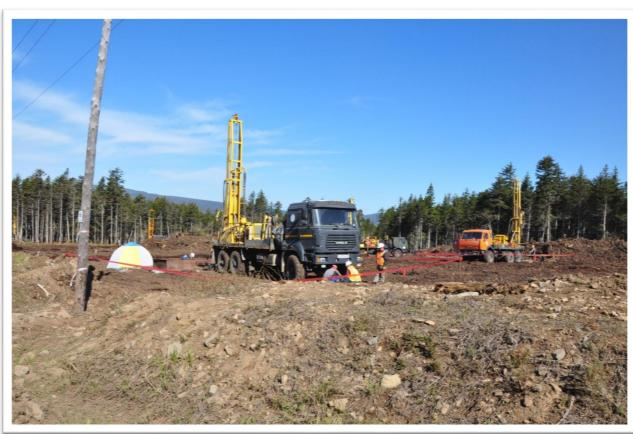
"URB 2A-2D" Exploration Drilling Rig on basis of "Kamaz-43114"
