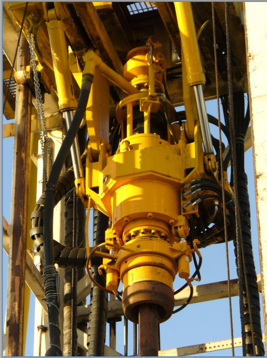
Power Swivel Wirth with hydraulic drive
